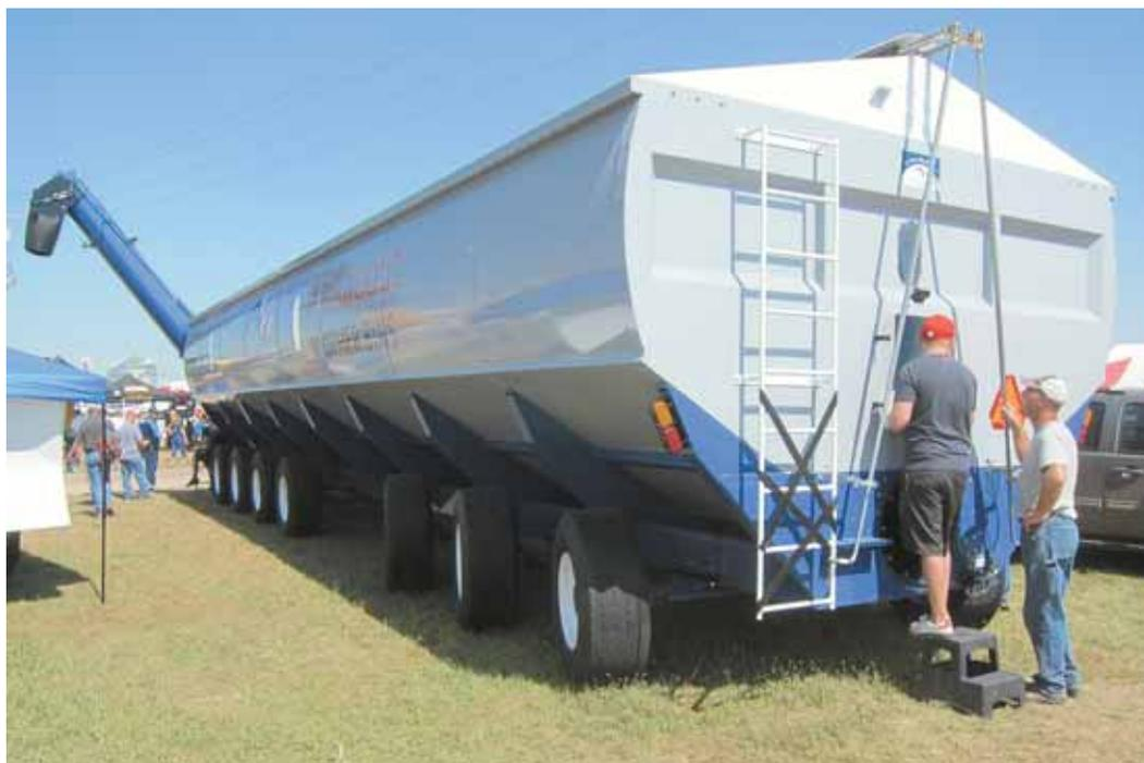
The Walkabout Mother Bin provides 4,000 bu. of in-field storage. “Instead of dumping grain into trucks directly, the grain cart operator fills the Mother Bin,” says Dave Hedt. “Trucks are then loaded from it. As a result, carts don’t have to wait for a truck, and trucks don’t have to wait for the cart to bring more grain from the combine.”
