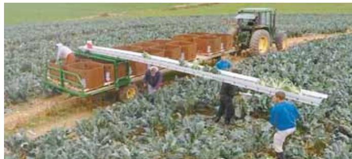
Proveyor wagon-mounted conveyor makes picking produce in the field a lot more efficient and is easier on the crew.
