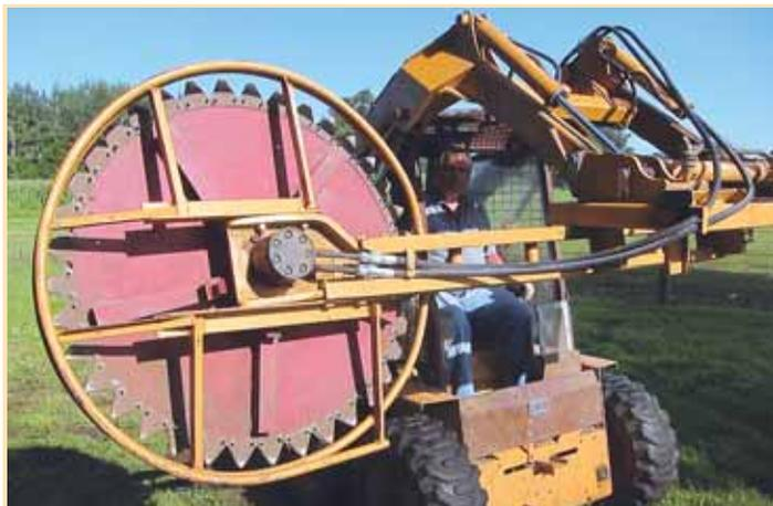
Giant cutter wheel uses mower sickle sections bolted around the perimeter of a 36-in. dia. steel plate to clear a 42-in. wide path. Plate is shaft-driven by a hydraulic motor.
