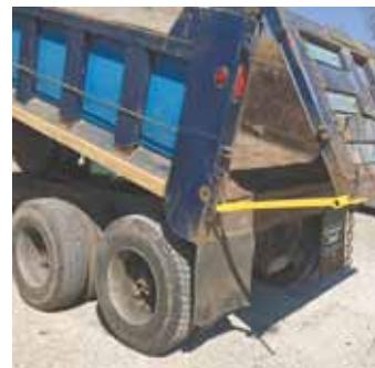
**Dump bed locks, left, hold truck bed securely in the "up" position. At right, Gate-Lok safety bar secures a truck endgate in the open position.**
