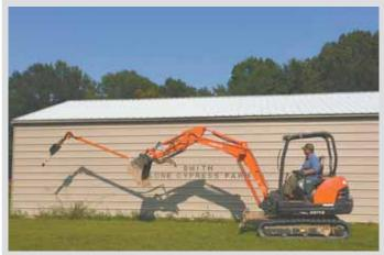
Instead of using his Limbinator hydraulic saw on a loader bucket, Verlis Smith mounted it on back of a Kubota backhoe bucket that he uses on his Arkansas farm.
