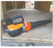
It only weighs 8 lbs, but with its 56V battery, it puts out up to 465 cfm with an air speed of up to 125 mph. Set it down while it's running and it will blow itself across the floor.
