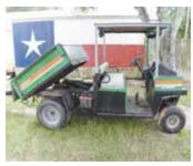
Joey McLennan, Edna, Texas: "I'm rebuilding an old Cushman truckster once used as a golf course utility vehicle. It's equipped with a 27 hp., 3-cyl. engine that purrs like a kitten. The company builds a high-belly dump box for it which I mounted on the rig's flat box. A single hydraulic cylinder raises and lowers the box and can handle loads up to 500 lbs.
