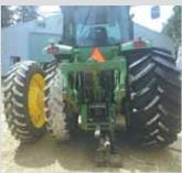
Lorn Manthey replaced the original R20/8046 rear duals on his Deere 8220 planter tractor (left) with new single LSW 900/50R46 tires. Even though he now plants directly into the tire tracks, there's less compaction than there was before in the "pinch row" between tires.
