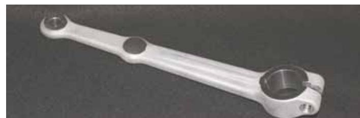
Eric Rego uses 3D machining to make replacement parts, such as the Oliver steering arm shown above.
