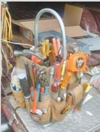
"Canvas-type tool holders designed to fit over a 5-gal. pail can hold a lot of tools, but because the bottom of the pail is round they can tip over easily."
