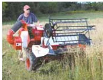
The Boaz weighs just over 900 lbs. and has 3 speeds forward plus reverse. It’s powered by a 13 hp. gas engine and measures 11 ft. long, 5 1/2 ft. wide and just over 4 ft. tall. The cutting platform is 30 in. wide. The operator rides on a seat over the rear dolly wheel operating controls similar to those on a 2-wheeled walk-behind tractor.
