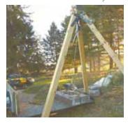
Menard (www.vispieux.com-tools; ph 819 829-2501). Works great for a variety of uses, but especially if I need to pick up heavy objects in out of the way places. The Smartripod hardware bolts to 4 by 4's that pin together, providing a 2,000-lb. lift capacity.
