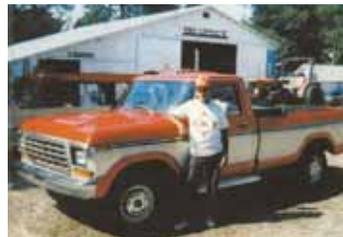
**Marion Klutzke, West Lafayette, Ind.:** In 1988 Klutzke bought a 1979 **Ford** 4-WD pickup that had been repowered with an Allis Chalmers 4-cyl., 200 cu. in. turbocharged and intercooled diesel engine equipped with a C-6 automatic transmission. The engine came out of an Allis Chalmers 6080 tractor.
