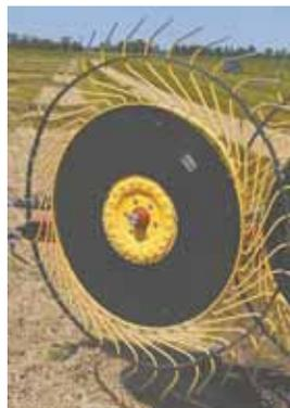
“After owning several wheel rakes over the years, we were getting real tired of replacing rake teeth all the time. So when we traded for a new rake we installed these bands right away. They reduce damage to rake teeth in rough conditions, and after a full season of use we haven’t had a single broken tooth. Not only does the rake run much quieter, it seems
