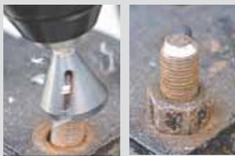
**Uniburr Tool Bit:** A new deburring tool makes it easy to repair bolts with damaged threads. It fits in a power drill and grinds down the end of a bolt, shearing off threads rather than folding them over as can happen with a grinder. The company says it doesn't "chatter" and won't overheat the work piece. The standard model sells for \$44.95 and is available at Amazon or www.uniburr.com (ph 800 864-2877). A Uniburr Plus model for harder steel sells for a bit more.
