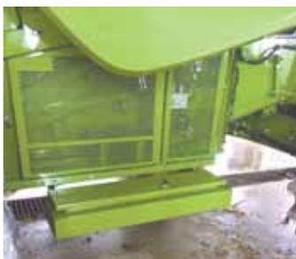
**Toolbox is 4 ft. long by 10 in. deep. It's designed to replace lower step on left side of combine.**
