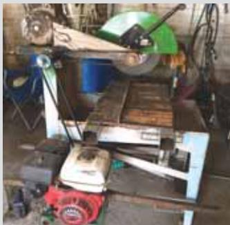
at an auction for \$20 and converted it to a portable steel-cutting choppersaw. The saw's electric motor didn't work so I replaced it with a Honda 9 hp gas engine. I also installed a new driveshaft and replaced the saw's belts and pulleys to fit."
