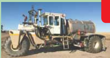
Floater Spray Rig Converted To Fire Buggy (Page 17)
