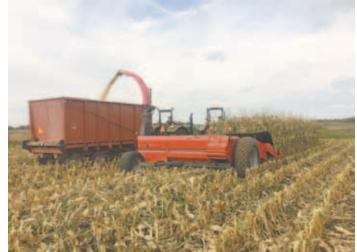
Marvin Bearinger's cob meal harvester was made from several differ- Crop enters from the cornhead through the feederhouse to a feeding ent components, including the cutterhead off a Deere 3960 pull-type auger, which pushes it into the cutterhead. Material then moves to silage chopper, a Case IH cornhead, and the feederhouse off a Case an impeller blower off a Dion forage harvester. IH combine.
