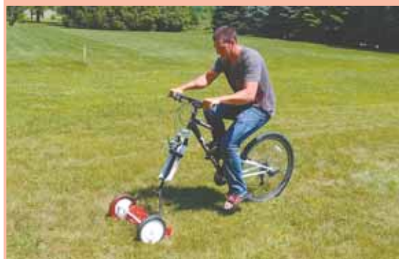
Bicycle's front wheel was removed and a bracket made that fastens reel mower to bike's wheel stem.
