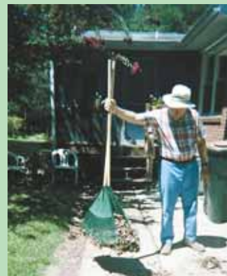
Wayne Carlton put 2 leaf rakes together facing each other and ran a long screw through both handles. The facing rakes work like giant salad tongs.
