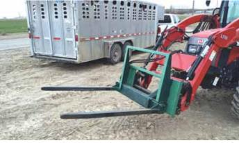
Loader-mounted bale fork uses a pair of squeeze arms attached to a steel backstop. One arm is stationary. An enclosed hydraulic cylinder moves other arm inward to grasp load.
