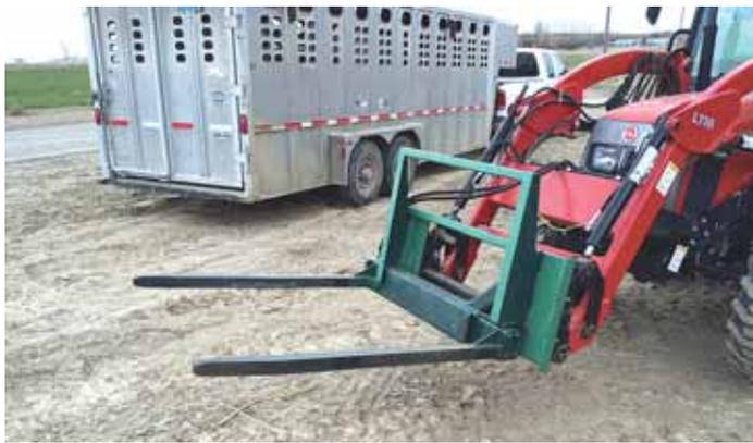
Loader-mounted bale fork uses a pair of squeeze arms attached to a steel backstop. One arm is stationary. An enclosed hydraulic cylinder moves other arm inward to grasp load.
