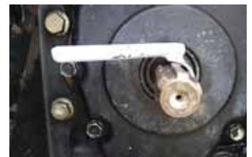
Pto alignment tool consists of a 4 1/2-in. long pipe that serves as a handle, with a sharply curved hook welded onto one end to grab a spline.
