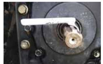
Pto alignment tool consists of a 4 1/2-in. long pipe that serves as a handle, with a sharply curved hook welded onto one end to grab a spline.
