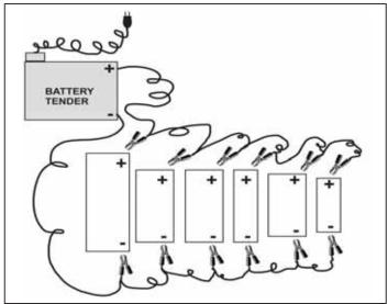
Norm Bennett came up with this low-cost system that uses a single trickle charger to maintain up to ten 12-volt batteries at a time.
