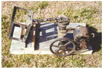
Automatic paint can shaker uses a 1/3 hp electric motor to belt-drive a right angle gearbox that reduces the speed.
