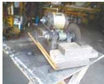
Herman Vander Vos puts worn metal cutting blades on his chopsaw, using a mandrel on an old belt-driven emery wheel as a mount for the blade.
