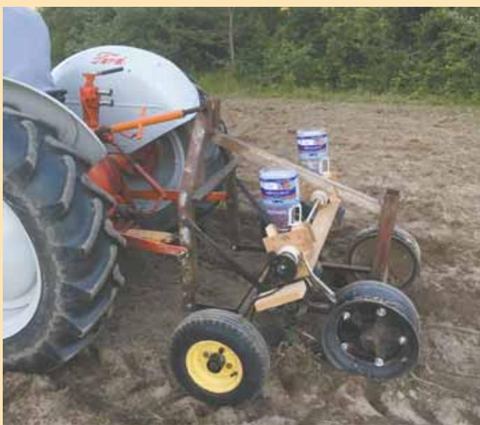
Rubber tire on planter's front axle drives a sprocket on a threaded rod axle on seeding unit (above). An adjustable wooden block serves as an idler wheel for the drive chain.
