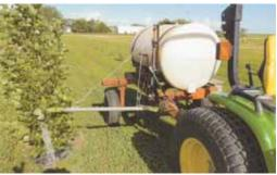
LaVern Peterson and relatives transformed a 300-gal. sprayer into this portable watering tank. When pipe is let down by cable attached to hydraulic cylinder, water gravity-flows out.
