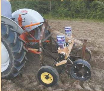
Rubber tire on planter's front axle drives a sprocket on a threaded rod axle on seeding unit (above). An adjustable wooden block serves as an idler wheel for the drive chain.
