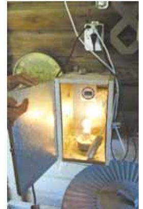
Fromelt built a wood box for an electronic timer and installed a 15-watt light bulb inside it to keep timer from freezing.
