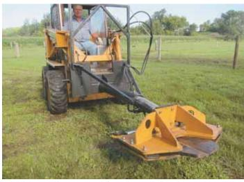
"It's built heavy so I'll be able to use it for years and years," says Mark Majerus about his skid loader-mounted tree shear. It's equipped with 2 fixed blades of 1-in. thick T100 steel.
