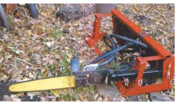
Skid loader-mounted chainsaw operates off the machine's hydraulics. It lets 93-year-old James Walsh still cut firewood even though he doesn't have the balance and strength to run a chainsaw.
