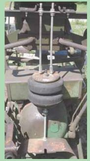
C. Roger Podoll made an air ride seat for his Oliver 770 using the airbag off a truck. It's mounted between tractor's pto shield and seat
