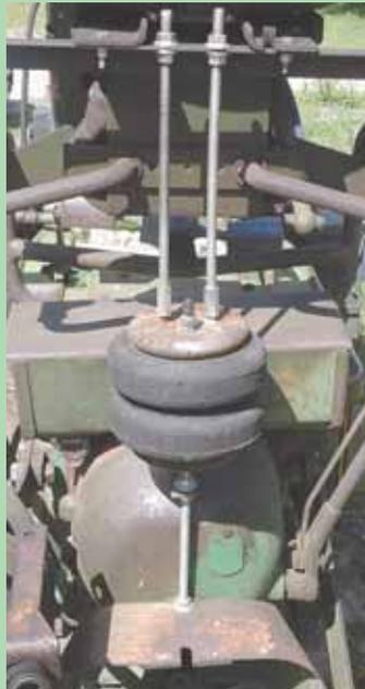
C. Roger Podoll made an air ride seat for his Oliver 770 using the airbag off a truck. It's mounted between tractor's pto shield and seat.
