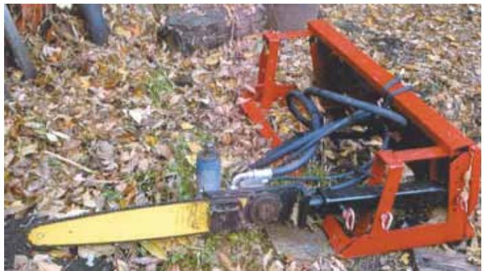
Skid loader-mounted chainsaw operates off the machine's hydraulics. It lets 93-year-old James Walsh still cut firewood even though he doesn't have the balance and strength to run a chainsaw.
