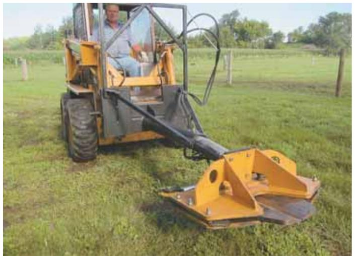
"It's built heavy so I'll be able to use it for years and years," says Mark Majerus about his skid loader-mounted tree shear. It's equipped with 2 fixed blades of 1-in. thick T100 steel.
