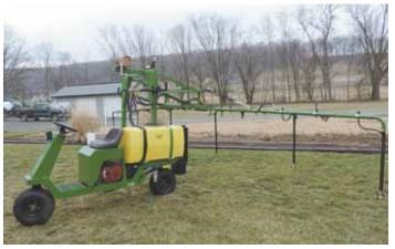
Self-propelled SP-50 sprayer comes with a 50-gal. tank and 22-ft. boom. It's powered by a 13 hp. Honda engine and has hydrostatic, single wheel drive.
