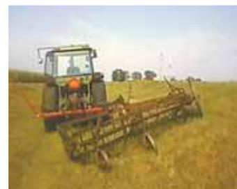
Folding 3-pt. toolbar attaches to a quick hitch and is used to pull an old hay rake. It lets Duane Johnson rake hay on roadside ditches while keeping his tractor on the level.
