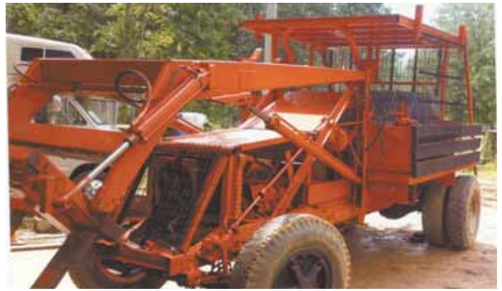
Boom lifts loads up to 20 ft. high, allowing Coleman to stack round bales up to 5 high inside his barn.
