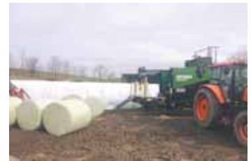
Norwegian-built Orkel stationary baler wraps chopped silage in plastic. Silage is dumped in by a loader bucket, compacted, and then wrapped.
