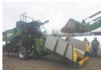
Norwegian-built Orkel stationary baler wraps chopped silage in plastic. Silage is dumped in by a loader bucket, compacted, and then wrapped.
