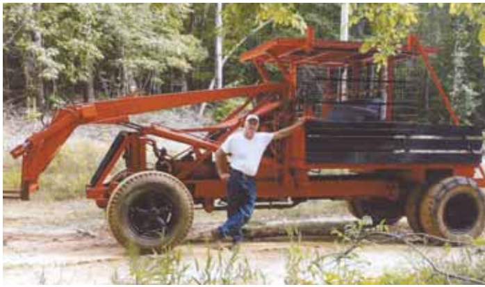
Jerry Coleman built this big loader tractor out of an old 65-passenger schoolbus. "It drives more like a car than a tractor," says Coleman.
