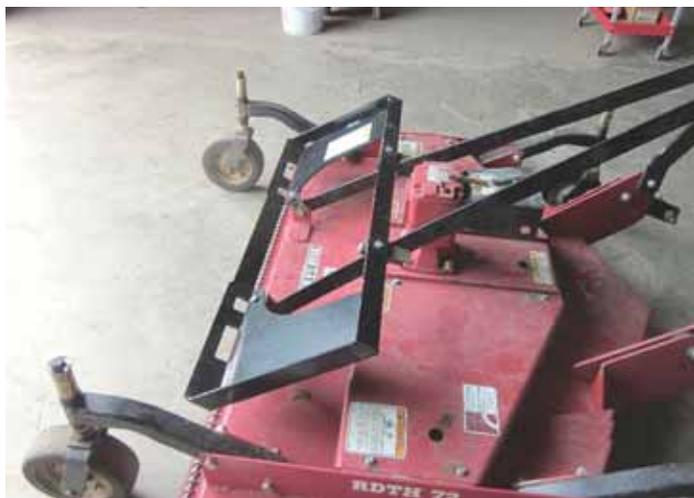
Darry Markle bolted a skid loader quick-tach universal mounting plate onto the deck of his 3-pt. mounted, 6-ft. finishing mower.
