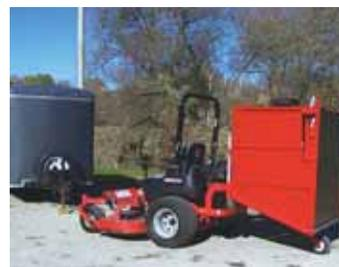
Clippings are blown into a small trailer that he built out of 1-in. tubing and plywood.
