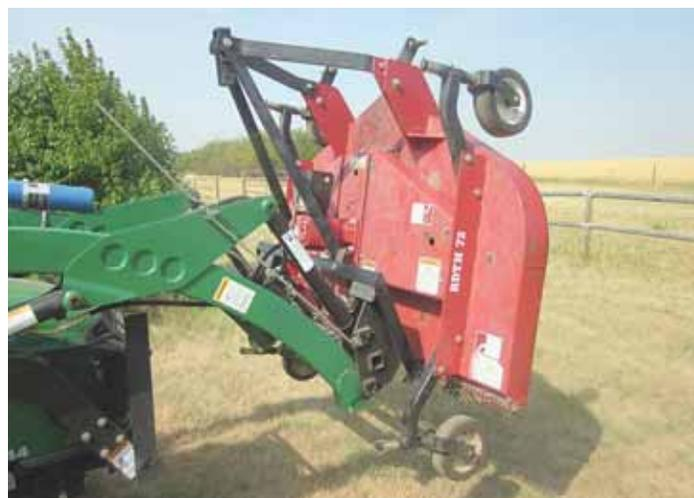
"It lets me disconnect the mower from the 3-pt. hitch and raise the deck up off the ground so I can service the blades safely while standing up," he says.
