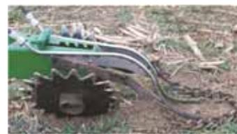
closing wheel bracket of a Deere or Kinze planter. It includes a Y adapter that fits the fertilizer supply line, laser cut tubes formed with a CNC bender, a weldment that bolts to each side of the closing wheel, and two 11-in. pieces of hydraulic hose. The kit doesn't include drag chain.
