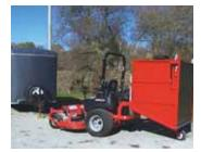
Clippings are blown into a small trailer that he built out of 1-in. tubing and plywood.
