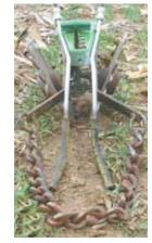
No-till farmer Alvin King and his sons built this Nutri-Placer kit that puts fertil-izer within 2 in. on both sides of the row for more uniform plant uptake. They recommend using it with drag chains.
