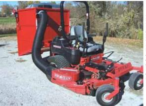
Leonard Mallas repaired a scrapped-out leaf blower vac and used it to build a high capacity collection system for his Gravely 60-in. zeroturn riding mower.
