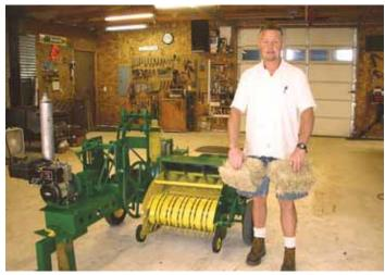
Patrick Burrington's 1/3-scale mini baler is modeled after old-time small square bale Baler makes compact 5 by 7 by 12-in. bales that average 6 to 7 lbs. presses made in the 1930's and 40's. It's driven by a 5 hp. gas engine.
