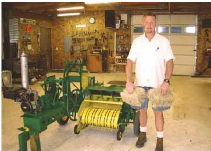
Patrick Burrington's 1/3-scale mini baler is modeled after old-time small square bale presses made in the 1930's and 40's. It's driven by a 5 hp. gas engine.
