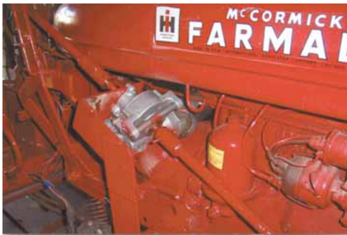
Ken Hall used the electric power steering motor from a car to add power steering to his Farmall "B". He cut 1 ft. out of tractor's steering shaft to attach motor.
