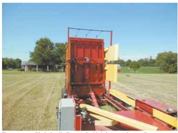
Floor on wagon lifts hydraulically to stacks 6-bale layers against a pallet.
