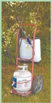
Eric Holmes mounted a propane torch flame weeder on a hand cart in order to control weeds on his property. A 4-gal. backpack sprayer mounted on back of cart is used for fire control.
