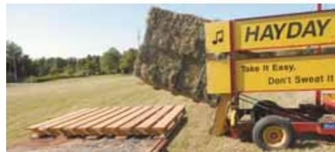
**Once pallet has 4 or 5 layers against it, wagon tilts pallet and bales 90 degrees and then sets loaded pallet onto a trailer.**
