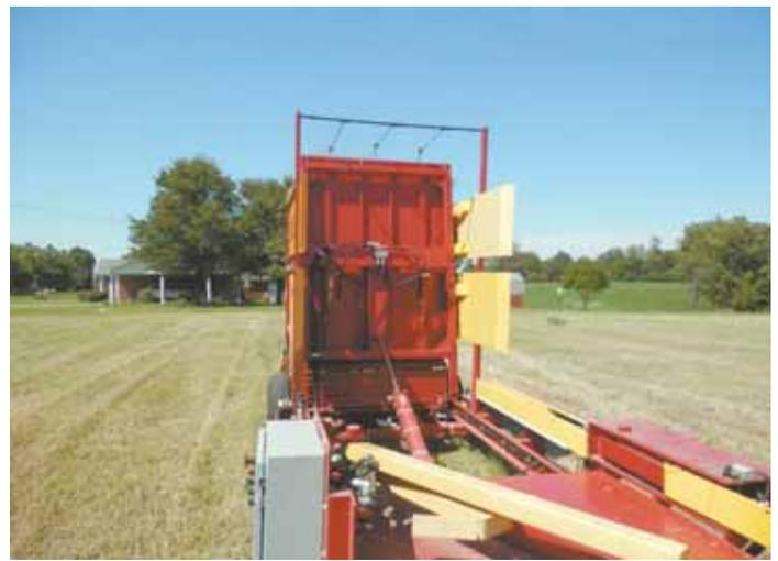
**Floor on wagon lifts hydraulically to stacks 6-bale layers against a pallet.**
