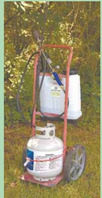
**Eric Holmes mounted a propane torch flame weeder on a hand cart in order to control weeds on his property. A 4-gal. backpack sprayer mounted on back of cart is used for fire control.**
