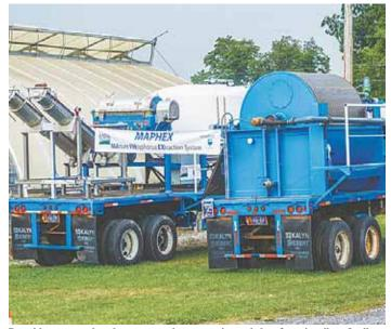
Portable manure phosphorus extraction system is carried on 2 semi trailers. It allows dairymen to use phosphorus for fertilizer or sell it as a value-added product.
