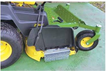
"It results in easier trimming and parking in tight areas," says Al Robbins, who replaced the grass discharge chute on his riding mower with this homemade "chain guard".
