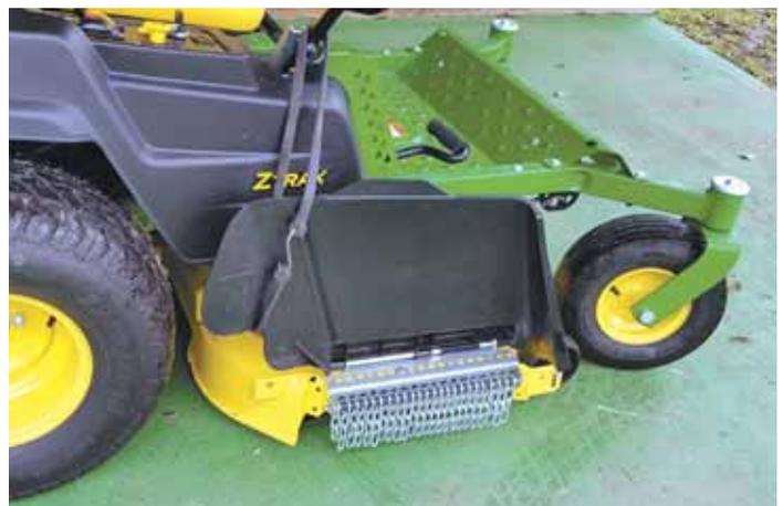
"It results in easier trimming and parking in tight areas," says Al Robbins, who replaced the grass discharge chute on his riding mower with this homemade "chain guard".
