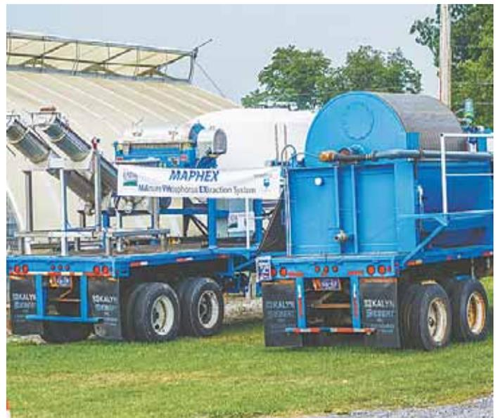
Portable manure phosphorus extraction system is carried on 2 semi trailers. It allows dairymen to use phosphorus for fertilizer or sell it as a value-added product.
