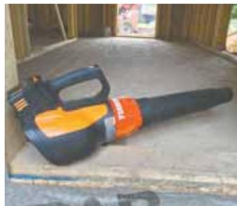
It only weighs 8 lbs, but with its 56V battery, it puts out up to 465 cfm with an air speed of up to 125 mph. Set it down while it's running and it will blow itself across the floor.
