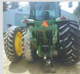
**Lorn Manthey replaced the original R20/8046 rear duals on his Deere 8220 planter tractor (left) with new single LSW 900/50R46 tires. Even though he now plants directly into the tire tracks, there’s less compaction than there was before in the “pinch row” between tires.**
