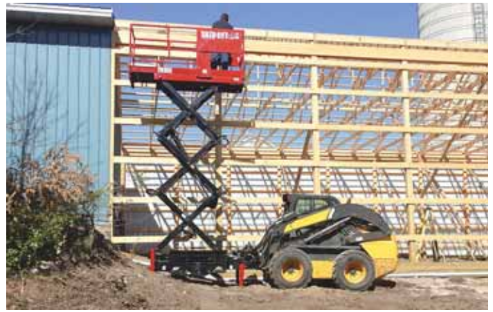
Each unit comes with telescopic legs, an anti-slip deck surface, and base controls with safety let-down valve and emergency stop switch.
