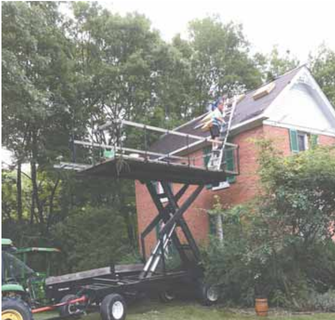
Jim Schintler started with a damaged scissors lift truck and ended up with this handy home-built lift. The roomy 8 by 14-ft. bed lifts a little more than 14 ft. high.
