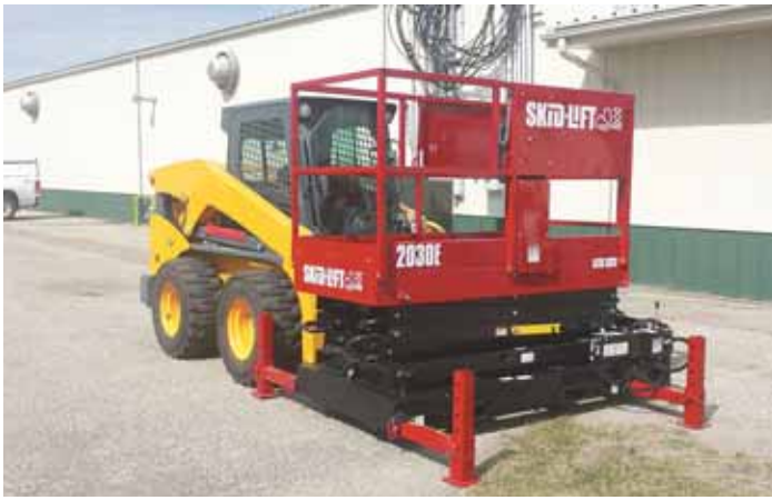
Scissors lift attaches to the quick-tach plate on any skid loader, taking advantage of loader's drive system, hydraulics, and steering.
