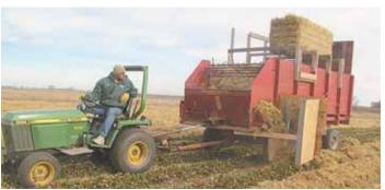
An old forage wagon spreads an even swath of straw on Dan Brouwer's strawberries. Wagon's extended discharge chute is the same width as a row of strawberries.
