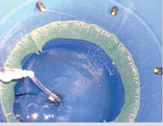
Shamburg built his "Swamp cooler" out of a 55-gal. plastic barrel with a fan on top that faces down into the barrel. A small pump pulls water out of the bottom of the barrel to side-mounted nozzles, which saturate "miner's moss" that covers 5 aeration holes cut into the side of barrel. Air is cooled as it passes through the wet material.
