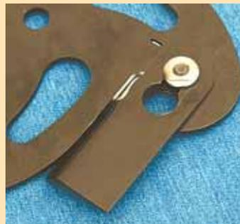
Closeup photo shows how blade tip slips over bolt head on bottom of blade so it's free to swing.
