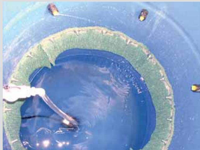
Shamburg built his "Swamp cooler" out of a 55-gal. plastic barrel with a fan on top that faces down into the barrel. A small pump pulls water out of the bottom of the barrel to side-mounted nozzles, which saturate "miner's moss" that covers 5 aeration holes cut into the side of barrel. Air is cooled as it passes through the wet material.
