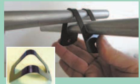
To use the clip you squeeze both ends and slip in pieces of conduit, and then release. Spring tension holds conduit tightly in place.
