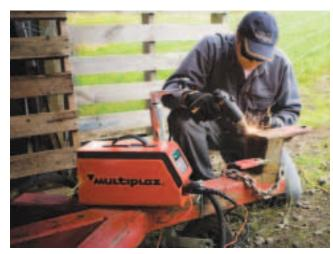
Not much bigger than an old-time radio, all the Multiplaz 3500 welder needs is 110 or 220-volt current, water and alcohol.
