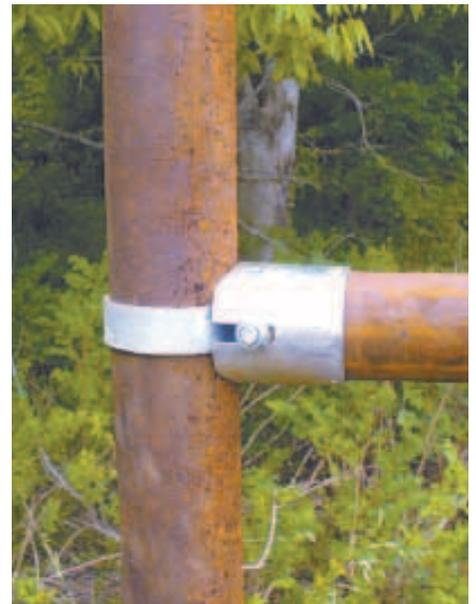
Pipe connector kit includes a band that clamps onto a 2 7/8-in. pipe post, and a double-slotted sleeve that slides over a 2 3/8-in. cross pipe. A carriage bolt runs through band.
