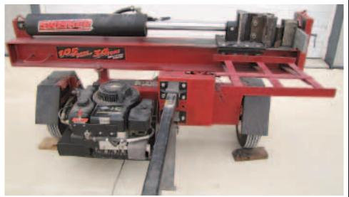
The metal is placed between the square block and the V-block, which is held in place by a steel back plate with a pair of guides welded onto it.
