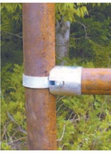
Pipe connector kit includes a band that clamps onto a 2 7/8-in. pipe post, and a double-slotted sleeve that slides over a 2 3/8-in. cross pipe. A carriage bolt runs through band.
