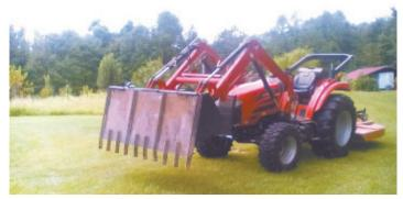
Blade is sized to match a standard 6-ft. bucket and drops about an inch below bucket's cutting edge. Teeth extend about 4 in. below edge of blade.
