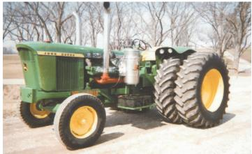
David Will replaced the locked-up engine on his Deere 5020 tractor with a Detroit V-12 diesel engine with about 450 hp. "I use it to pull a 30-ft. field cultivator. It's really loud," says Will.
