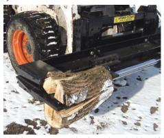
Multi-purpose machine is equipped with a 10in. tall, 4-way splitter blade with the vertical part welded to boom. Splitter's cross blade is bolted on.
