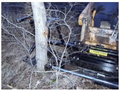
By unbolting cross blade and bolting a push bar/catcher onto boom, operator can shear trees, catch them, and haul them away (above). Boom can also be used to prune tree limbs up to 16 ft. high.
